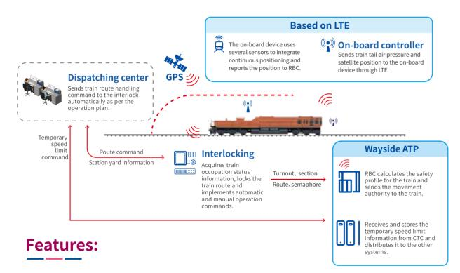
Integrates LTE technology with train-to-ground communication. Uses satellite navigation technology for train positioning. Safety brake model based on heavy haul railway.
