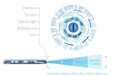
In the new generation Train Intelligent Detection System (TIDS), laser radar, vision and other sensor technologies are used to detect and protect the front line of the train along with using the intelligent algorithm of deep learning. Calculate the safe travel distance according to the train running speed, and carry out overspeed protection. Ensure the safety of the train and the operation efficiency of the line under emergencies.
